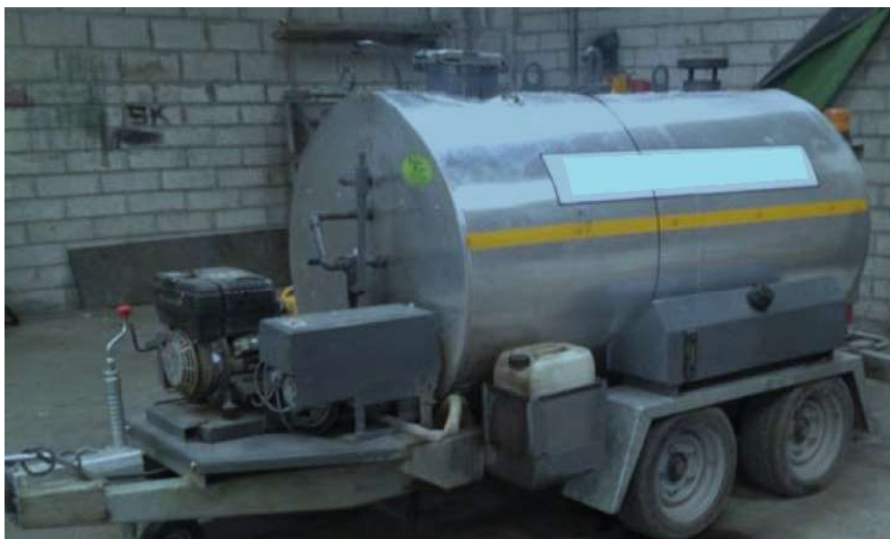
Figure 3-16: Towable Sprayer for Temporary Reinstatement
